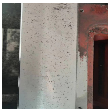
Nitrogen Porosity Morphology 氮气孔形态
