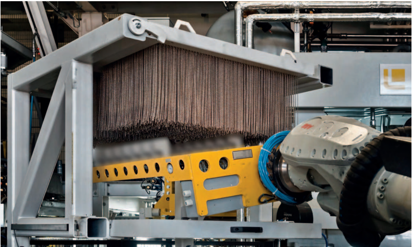
Core production is supported by eight Laempe automated cells, with advanced digitalization, making the company a pioneer in Core Production 4.0.
