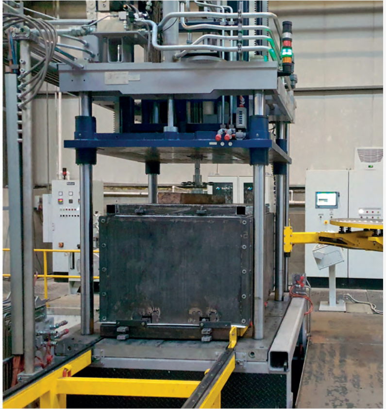
Highest flexibility for jobbing foundries: Kurtz AL13-13SC "2 in 1 Solution" – left side: permanent mold, right side: sand mold/core package
